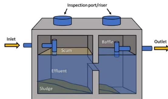
Figure 1. Illustration of a septic tank. Fats, oils, and grease that make up the scum layer float on the top, while heavier solids that make up the sludge settle to the bottom. This allows effluent water to leave the tank and enter the drainfield where it is treated by the soil.
